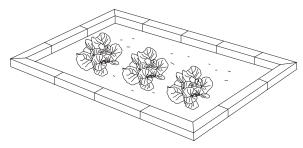
Cut two planks of wood, one to around 12 inches (30cm) in height and the other to around 20 inches (50cm) in height. Their lengths will be determined by your window. Then cut two more planks, for the sides, using the same measurements (12 & 20 inches) in order to create a slightly angled frame.
