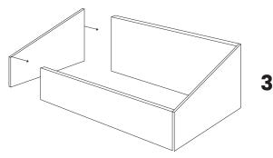
Nail or screw the planks together. You can also place small pieces of wood at the corners to reinforce your frame. The more solid, the better.
